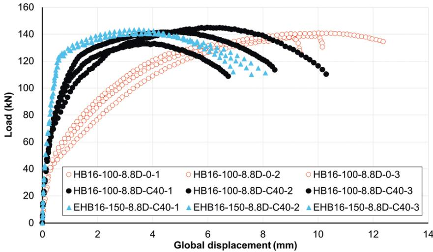
**Fig. 2** Pull-out behaviour of EHB in comparison with type HB with and without infill concrete [25] (specimen key: bolt type–bolt diameter–shank length–bolt grade and batch concrete grade–sample number)
