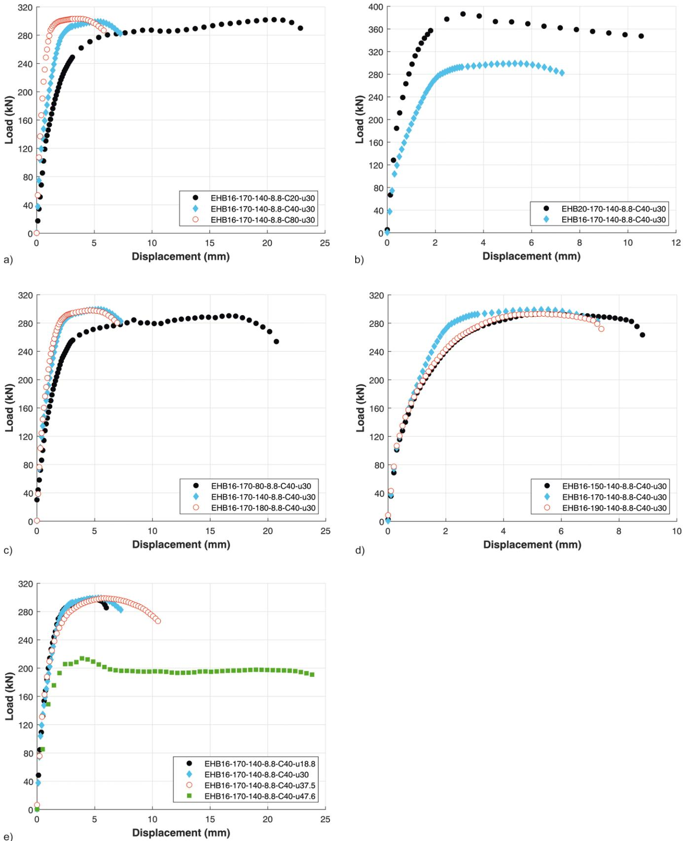
**Fig. 4** Experimental results for a) concrete samples C20, C40, C80, b) bolt diameter samples M16, M20, c) gauge distance samples G80, G140, G180, d) shank length S150, S170, S190 and e) tube wall slenderness ratio samples  $\mu 18.8$ ,  $\mu 30$ ,  $\mu 37.5$ ,  $\mu 47.5$  (specimen key: bolt type–bolt diameter–shank length–bolt grade and batch concrete grade–sample number)
