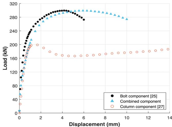
**Fig. 5** Bolt, combined and column components global vs. load curves for samples with concrete grade 40 MPa, bolt diameter M16, anchored length 80 mm, tube wall slenderness ratio 37.5 and gauge distance 140 mm
