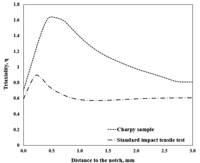
**Fig. 2** Triaxiality comparison between Charpy sample and standard impact tensile sample
