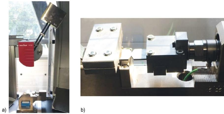
**Fig. 1** a) Impact pendulum with new hammer for tensile impact test, and b) clamping system with fixed specimen
