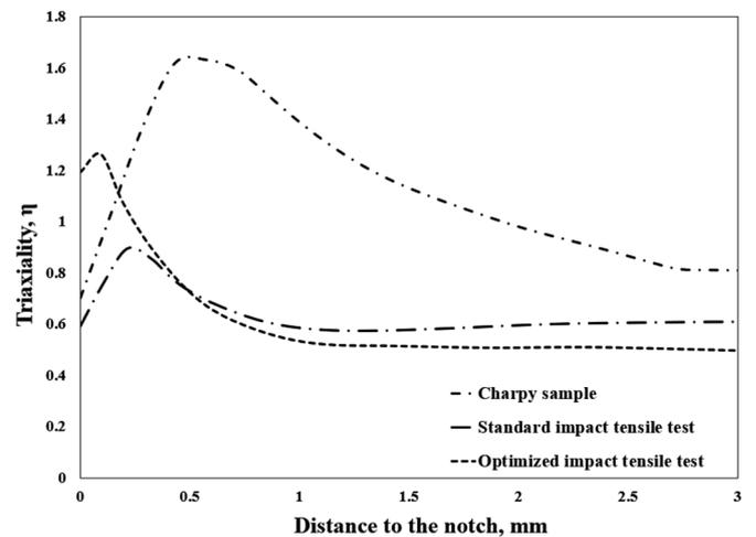
**Fig. 5** Triaxiality comparison between Charpy sample, standard impact tensile sample and optimized impact tensile sample
