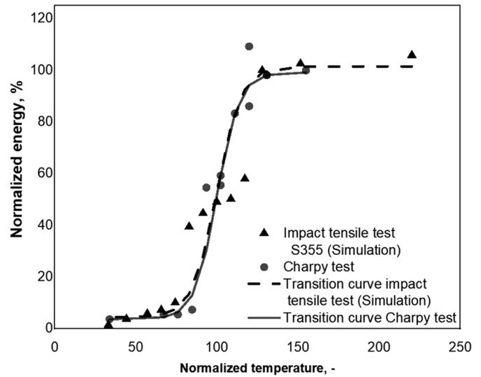
**Fig. 6** Correlation between the transition curves of Charpy tests and impact notch tensile tests
