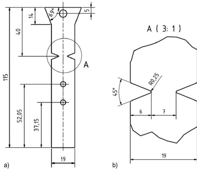
**Fig. 3** Standard geometry of impact notch tensile test specimen: a) overall view and b) detail view of notch, 1.5 mm material thickness
