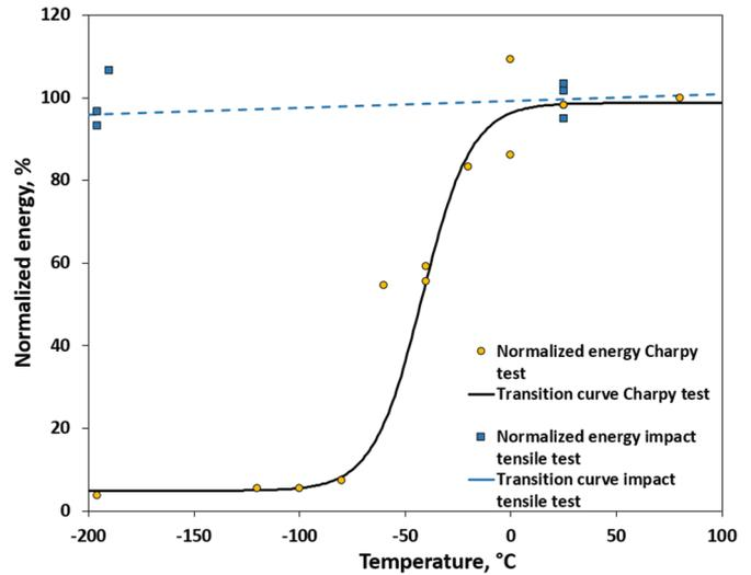
**Fig. 4** Normalized energy from experimental Charpy test and impact notch tensile test with the support of FE simulation
